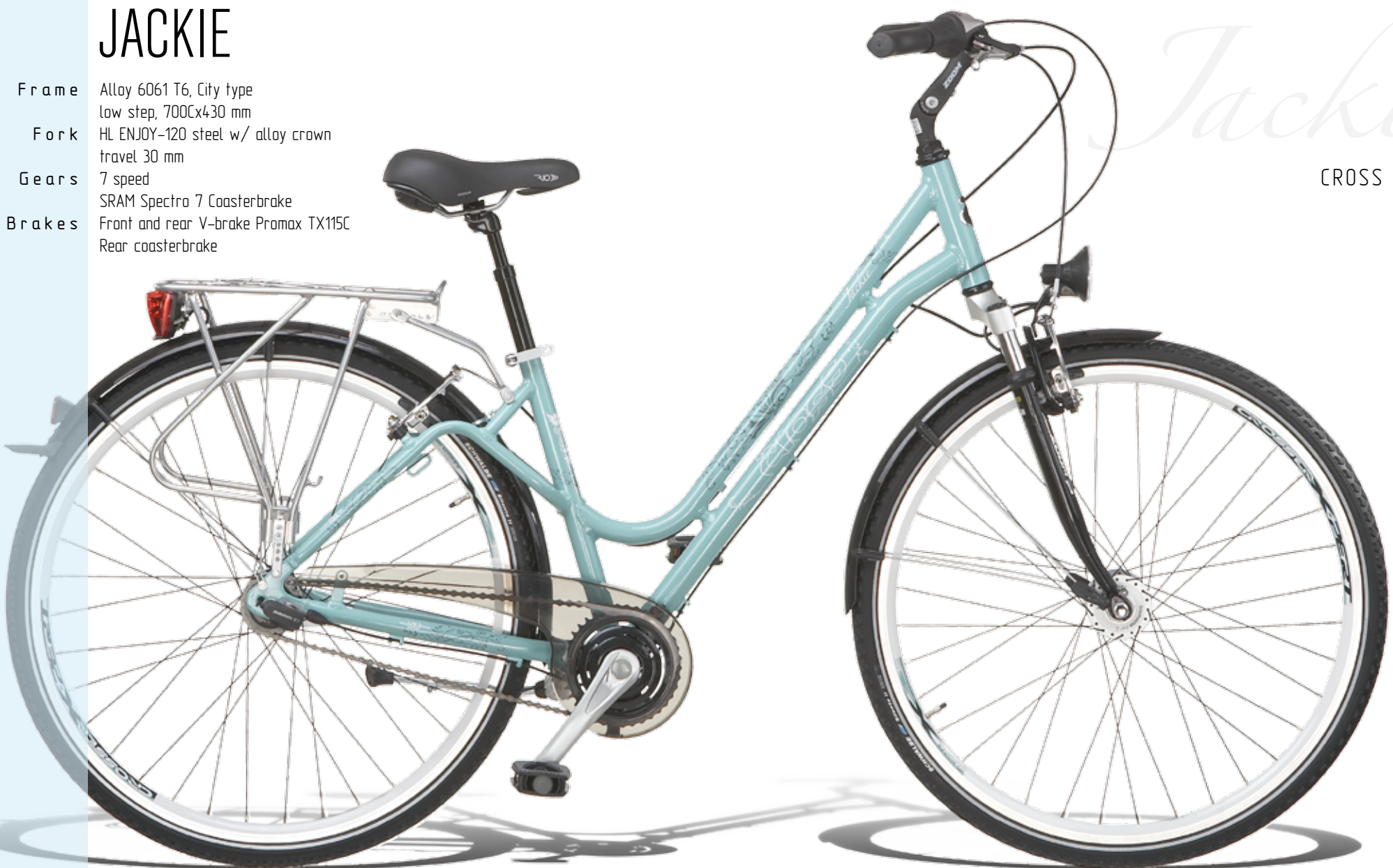
Wheels: Crosser X-PERT, alloy double wall profile - X3, 36 black spokes
