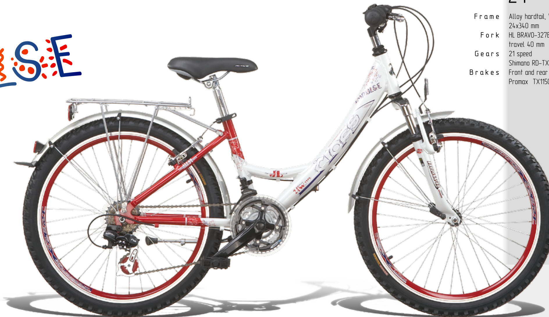
Wheels: Crosser X-PERT, alloy double wall profile - X3, 36 CP spokes
