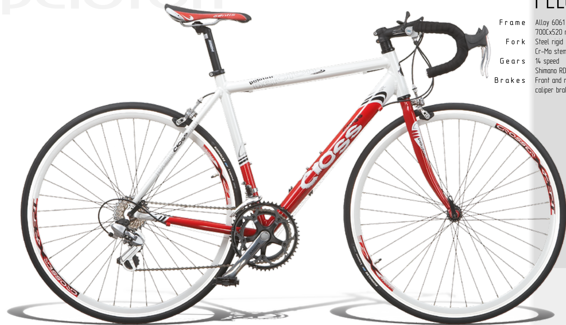
Wheels: Crosser X-PERT, alloy double wall profile - X4, 36 black spokes
