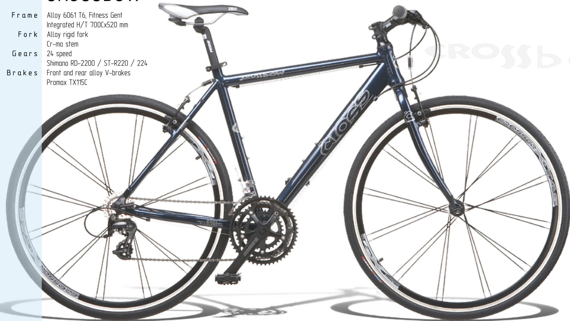
Wheels: Crosser X-TAS, alloy double wall profile - X4, 24 Aero black spokes 14G
